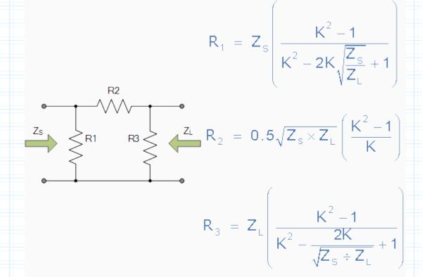
where: K is the impedance factor, ZS is the larger of the source impedance and ZL is the smaller of the load impedances.
