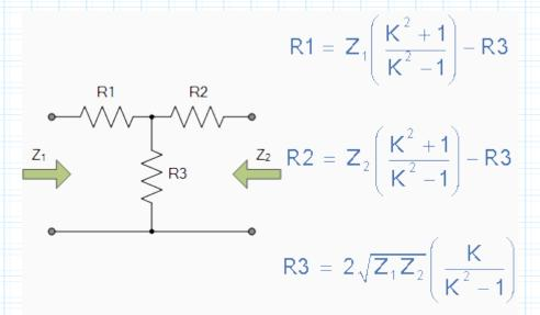
where: K is the impedance factor from the table above, and Z1 is the larger of the source/load impedances and Z2 is the smaller of the source/load impedances.
