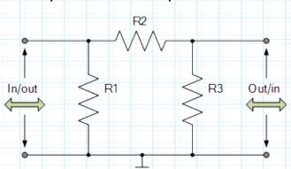
Generally, resistors R1 and R3 are of the same value but when designed to operate between circuits of unequal impedance these two resistor can be of different values.
