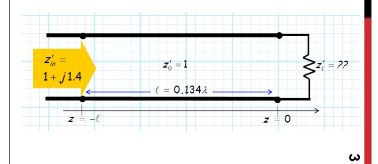
Q7 : A load terminating at transmission line has a normalized impedance zL' = 2.0 + j 2.0. What should the length I of transmission line be in order for its input impedance to be:
