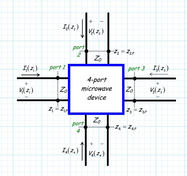
Note in this example, there are four identical transmission lines connected to the same "box". Inside this box there may be a very simple linear device/circuit, or it might contain a very large and complex linear microwave system.
