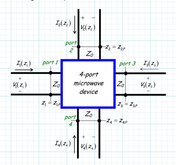
In addition to the Impedance Matrix, we can fully characterize this linear device using the Admittance Matrix.
