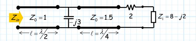
Note the resistor is in **series** with impedance  $Z_1$ . We can **combine** these two into one impedance defined as  $Z_2$ :
