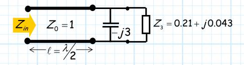
Now we find that the impedance  $Z_3$  is **parallel** to the capacitor. We can **combine** the two impedances and define the result as impedance  $Z_4$ :
