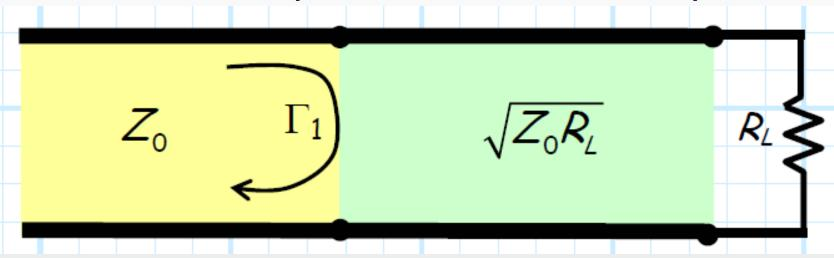
$\Gamma_1$  = **partial** reflection coefficient of a wave incident on the  $z = -\ell$  interface from the  $Z_0$  line:
