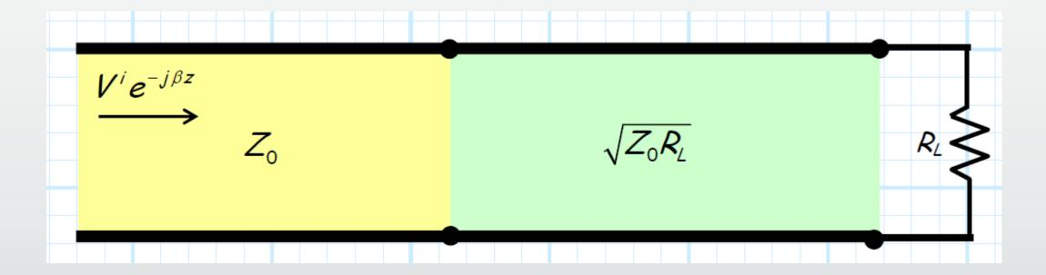
1. At  $z = -\ell$ , the characteristic impedance of the transmission line changes from  $Z_0$  to  $Z_1$ . This mismatch creates a **reflected** wave:
